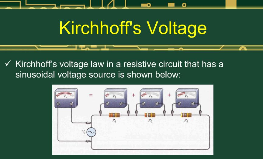
✓ The source voltage is the sum of all the voltage drops across the resistors, just as in a dc circuit.
