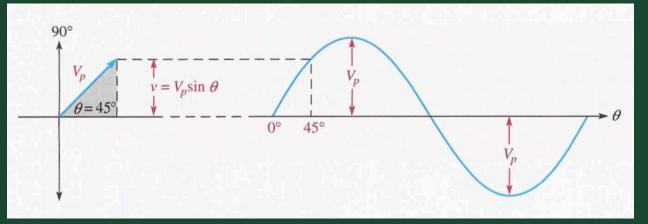
The vertical distance from the phasor tip down to the horizontal axis represents the instantaneous value of the sine wave at that point.
