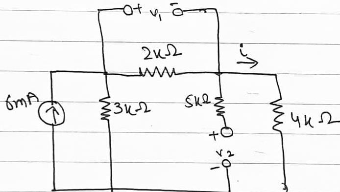
The current through the series combination of the  $2\text{k}\Omega$  and  $4\text{k}\Omega$  resistors is obtained by current division as:
