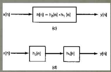
$$y[n] = w[n] * h_2[n] = (x[n] * h_1[n]) * h_2[n], \quad fig(a)$$
