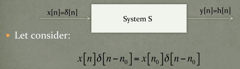
Representation of Discrete-Time Signals in Terms of Impulses (cont.) • Using the above fact we get the following equalities:  $x[n]\delta[n] = x[0]\delta[n], (n_0 = 0)$  $x[n]\delta[n-1] = x[1]\delta[n-1], (n_0 = 1)$  $x[n]\delta[n-2] = x[2]\delta[n-2], (n_0 = 2)$
