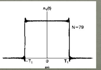
Fourier Series Representation of Discrete-Time Periodic Signals
